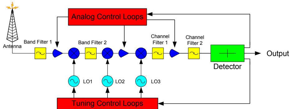
Figure 2: Traditional Super-heterodyne with analog detection
