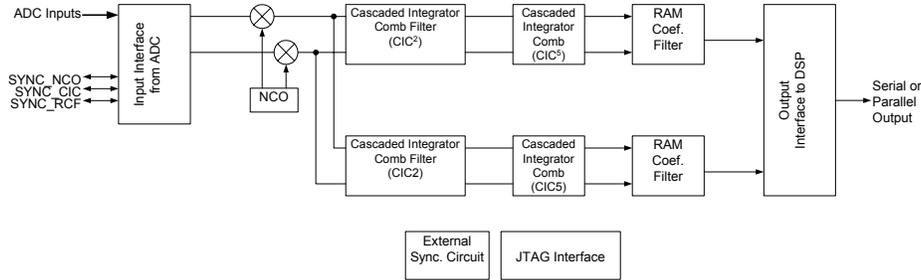
Figure 13: Fixed Function Receive Signal Processor (RSP)
