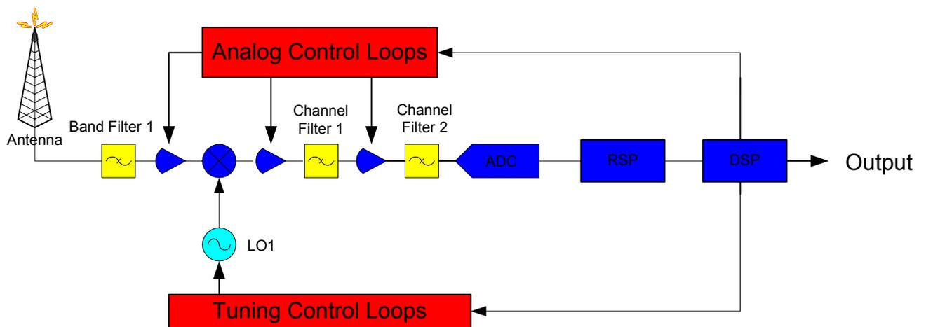
Figure 8: Single Carrier Rx Example
