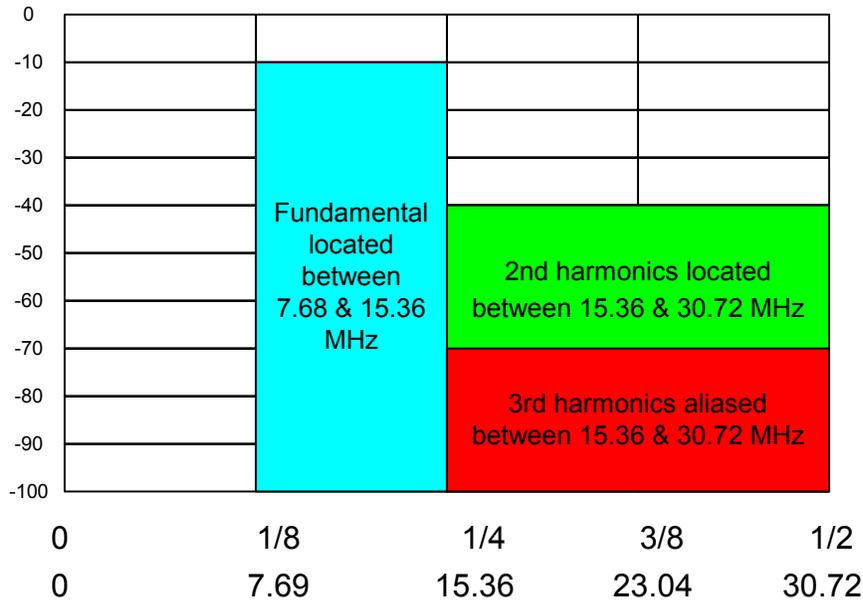
Figure 11: Aliased wideband signal and harmonics
