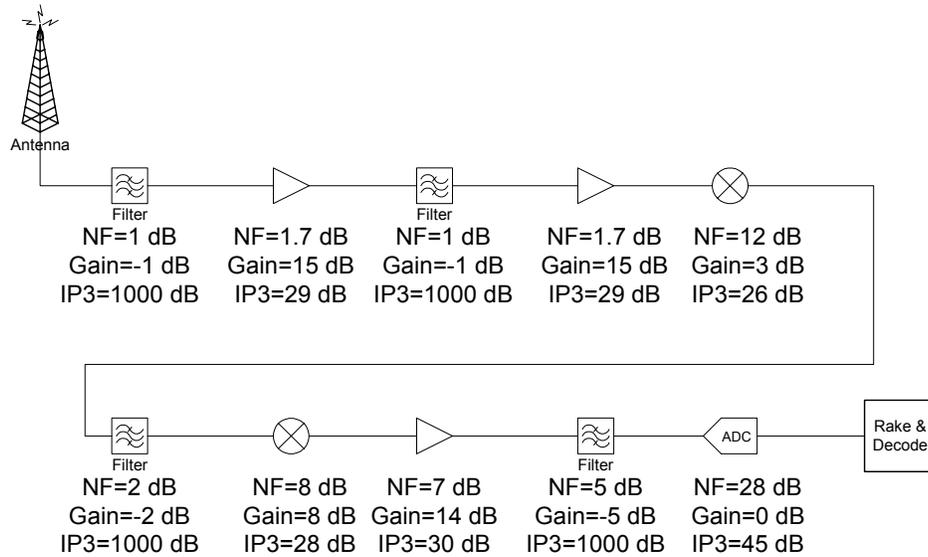
Figure 16: SDR receive signal chain
