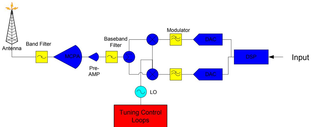
Figure 10: Single carrier direct conversion transmit
