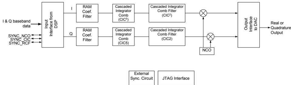
Figure 14: Fixed Function Transmit Signal Processor (TSP)
