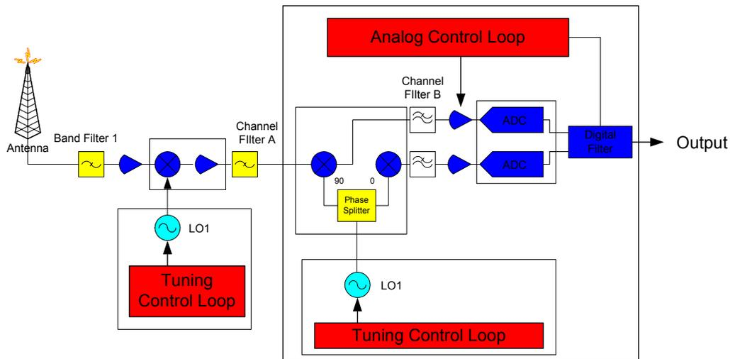
Figure 3: Super-heterodyne with baseband IQ sampling.
