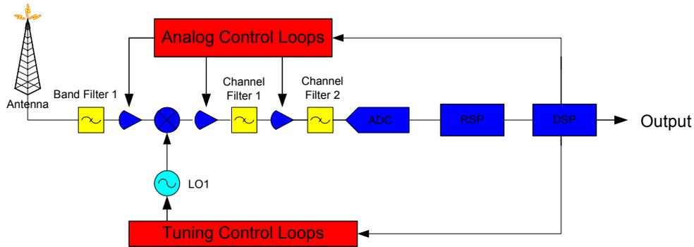
Figure 4: Super-heterodyne software defined radio
