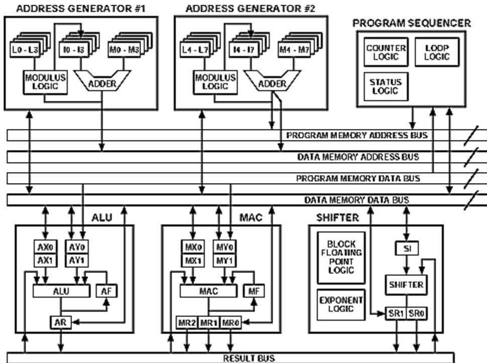
Figure 15: General Purpose Digital Signal Processor (DSP)
