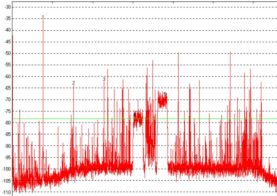
Figure 7: multi-mode spectrum with IS-95 and narrowband carriers
